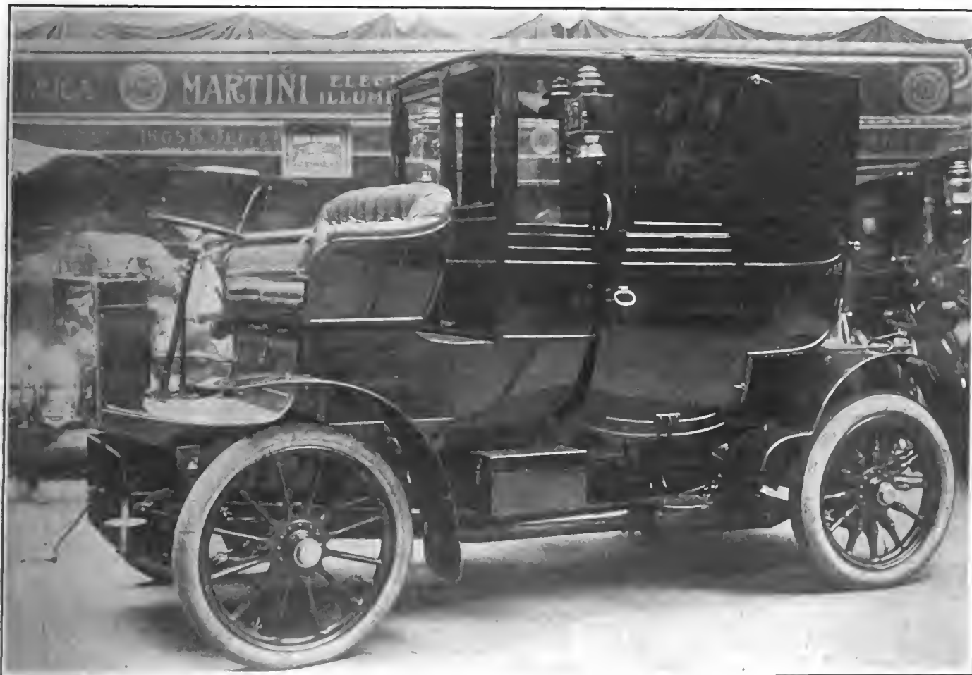
C. G. V. 25-HORSEPOWER ENCLOSED CAR FINISHED IN GREEN AND BLACK WITH MOTOR UNDERNEATH DRIVER'S SEAT.
